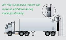
When a stationary head pad and wear pleat system is utilized, after time, movement of the trailer causes damage and can lead to detachment resulting in an unprotected wall surface and loss of seal
